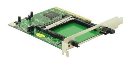
This PCMCIA PCI card gives you a PCMCIA slot on the back of your PC. The PCMCIA transfer rate is 16 bit (PC-Card) and 32 bit (Card Bus), supply voltage is 3.3V or 5V. The advantage of this PCMCIA PCI card is that you can use additional PC-Cards or card bus PCMCIA adapters like Wireless LAN, Bluetooth, USB adaptor, Firewire adapter, card reader, 10/100 LAN, etc. on your PC.
